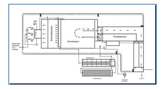
The influent of the fixed bed reactors amounts to a maximum of 20 m<sup>3</sup> of water per hour, which after successful biological purification is first stored in a retention basin and, after analytical inspection and approval, is conducted into a body of flowing water.
